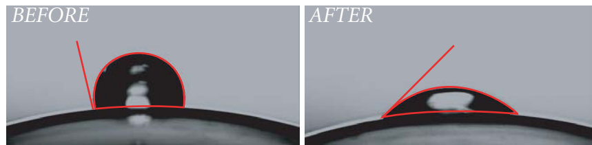
Contact angle measurements* of an RGP contact lens before and after plasma treatment.
