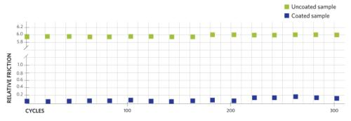
Coated polyurethane samples were pulled though a close-fitting PVC loop filledwith water. Force measurements were made after every 20 push/pull cycles.
